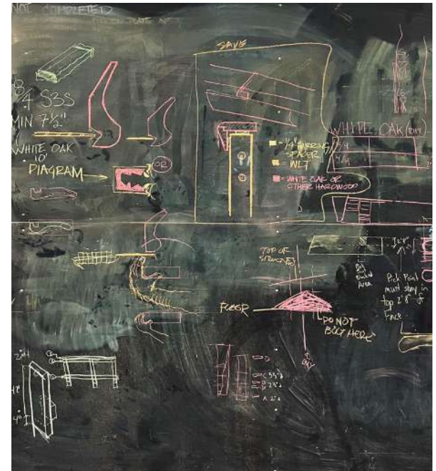
Example of student work - Initial sketches exploring intentions for the door jamb detail.
