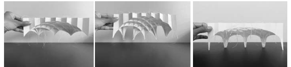
(Left) 1/4- scale muslin mock-up of canopy. Tension, fabric connections, and wind tests were conducted at the beach.
