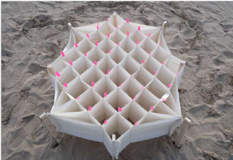
(Left) 1/4- scale muslin mock-up of canopy. Tension, fabric connections, and wind tests were conducted at the beach.
