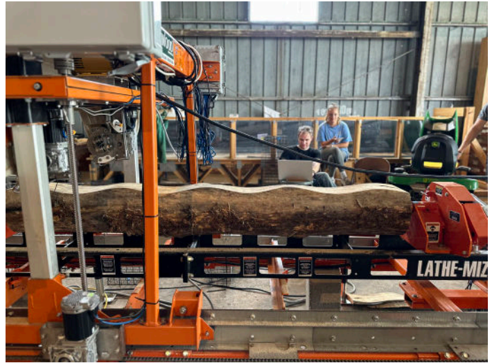
Robotic sawmill developed by a team led by Schumann at UVA. This technology is fully operational as of summer 2023. Students will be introduced to, trained on, and have access to the technology for fabricating material prototypes in studio.
