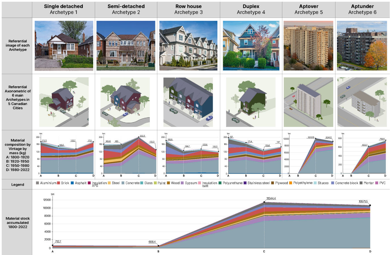
Figure 2. The average material composition of Canadian cities' residential buildings by archetype and vintage. Each archetype has a different scale, and the total accumulated material stock is presented at the bottom.
